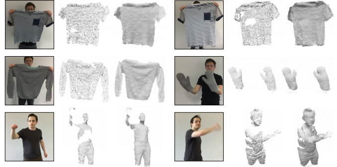
Fig. 8. Dynamic reconstruction on MPC-DD dataset by accumulating the input point clouds. Left: RGB image of the reference frame ( ref ), which are not taken as input. Middle: Unprojected depth point cloud from ref . Right: Accumulated points by warping other 3 frames to ref .
